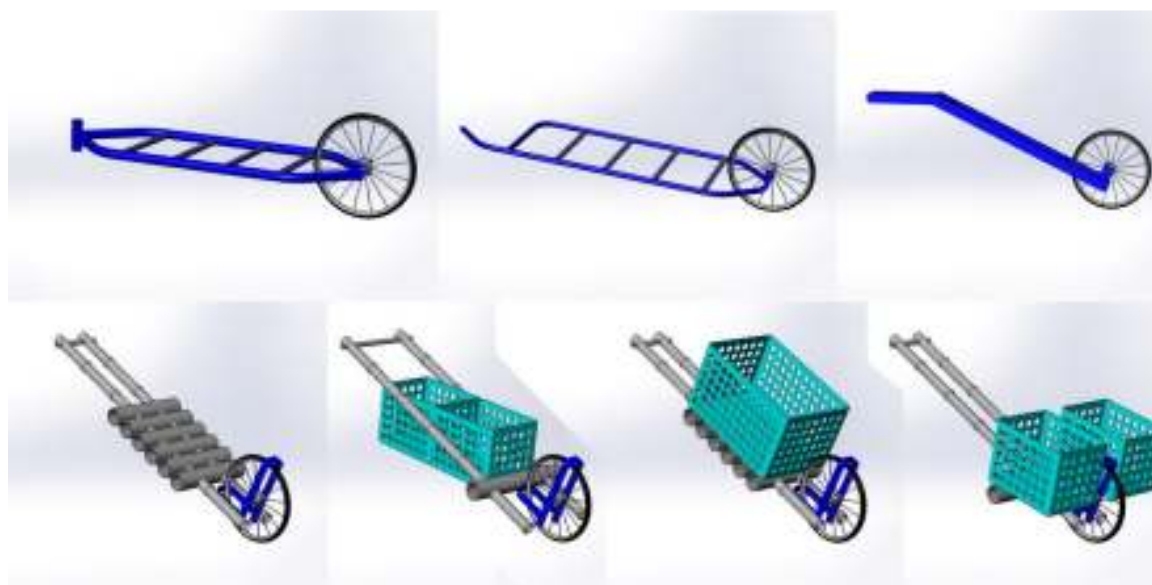
Designs of Bicycle trailers with one wheel, with metal (dark blue), bamboo (grey) and plastic (light blue) parts
