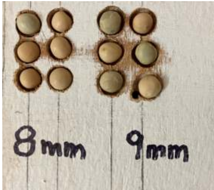
Braille Educational board, with dried peas representing large Braille dots The 8 mm and 9 mm are the diameters of the drilled holes
