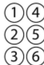
Figure 1 - Numbering the dots in Braille
