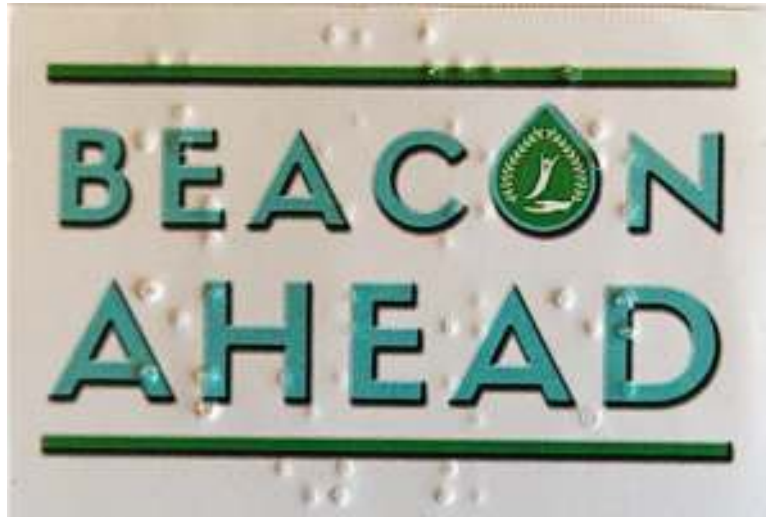
Figure 8 - Braille Printing on a 170 GSM visiting card
